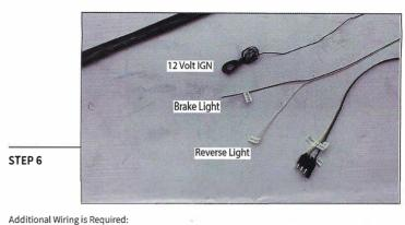
Brown (Brake) White (Reverse) Black (+ Transformer) Factory 12volt Brake Light Factory 12volt Reverse Light Factory 12volt Ignition wire
