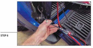
Next, with the key on and ENGINE OFF, apply the emergency brake and place the gear selector in reverse. Using a test light or multimeter, locate the 12volt power supply for the factory reverse light. Using the supplied scotch lock connector, connect the White wire from the tailgate light to the factory reverse light wiring.
