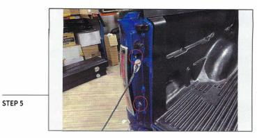
Additional wiring will require access to the factory tail light wiring. Begin by removing the fasteners that hold the tail light to the vehicle.
