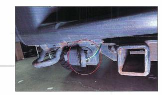
Wiring- Route the 4 pin plug so that the extra wiring is out of the way, and plug it into the factory plug. Then, run the black, brown, and white wire towards the tail light.
