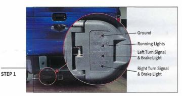
Begin the installation by locating the factory 4-Pin tailer plug. Using test light or multi-meter, test the trailer plug for all functionality; turn signals, running lights, and brake lights. If the plug isn't getting power, reference your owners manual to locate and test the trail plug fuse.
