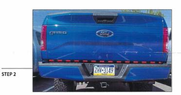
Next, locate a suitable mounting position for the light bar. Typical installation is between the tailgate and the bumper. Preparation for installation; thoroughly wash and dry the mounting location using an automotive grade soap and water. Ensure that you give the surface enough time to dry prior to installing the light bar. It is recommend that you wipe the mounting locations with isopropyl alcohol to ensure a wax and grease free mounting surface. \*\*Do not use silicone based cleaners.
