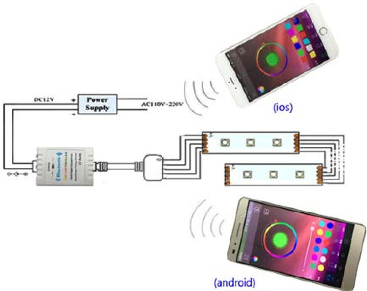
1. Only an input voltage of 5-24v DC can be used to power this controller, and the load must have the same voltage rating as the supply. Supplying a lower or higher voltage than the range of the controller and load may damage the controller and/or connected components.
