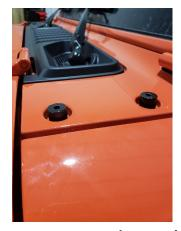
**3.** Once the brackets are mounted on the hood you may mount light bar to the hood brackets. Run the wire through the crevasse between the fender and wiper cowl of the vehicle.
