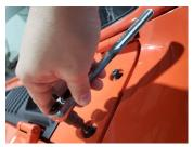
**2.** Use supplied bolts and spacers to mount brackets on wiper cowl on the hood of the vehicle. Do not tighten the bolts hand tighten only for now.
