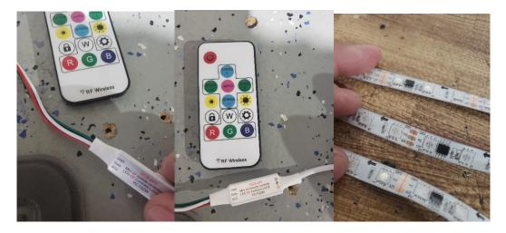
When cutting and soldering wires make sure pattern, arrows are facing the same way if one strip pattern arrow is backwards the chasing feature and the strips would not function properly and would be stuck on one color only. Wires from module are as follows Red is 12volts, White is Ground, Green is data for the patterns.
