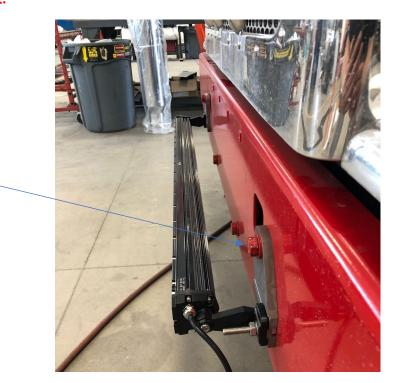
5. Assemble the light bar with Universal L-brackets with supplied hardware.
