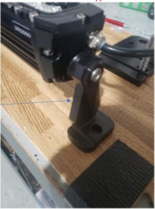
6. Align assembled light bar with bolts from bracket that is attached to bumper and assemble them with bolt washer supplied with kit. Once it is aligned secure and tighten all bolts and screws down.
