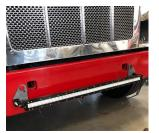
7. Finally wire up the supplied relay harness in the kit for the light bar. The output of the harness in Plug-n-play to the light bar connector. Wire 12+ volt power and ground to the harness and mount the switch in the desired location. You may need to extend the wires to the switch depending on your desired mounting location.
